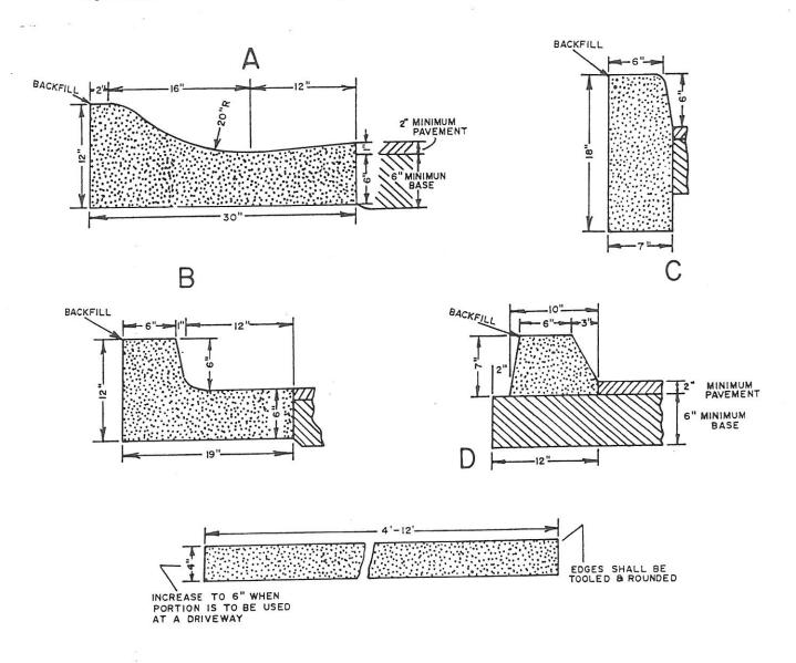
Type A. Base two (2) feet narrower than required pavement width.
